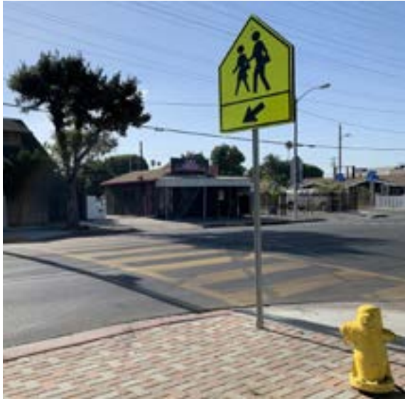
A ladder crosswalk with pedestrian crossing signage
